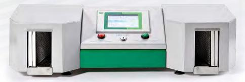
The FCM-02 monitor enables the measurement of the surface contamination of radiation workers, their clothing and working instruments by alpha, beta and gamma emitting radionuclides (depending on the detectors used).
